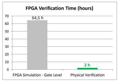
*Execution of all the FPGA verification procedures: 64.5 hours via logic gate level simulations VS 2 hours via physical tests. The time saved is around a factor of 30.*
