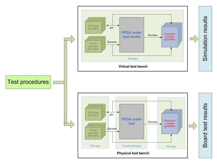
The virtual test bench and the physical test bench both allow the same inputs and generate the same type of output data. The test procedures can hence be written for both.
