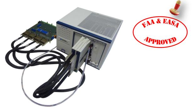
The NI test set consists of a PXI-1073 chassis with two PXIe-7962R modules combined with two NI 6581 adapters. With an acquisition frequency up to 100 MHz, they allow monitoring of various FPGA input and output signals.
